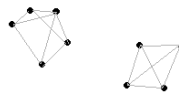
Fig. 5. Above is an kNN (undirected) graph of some graph G . Each node is connected with its three nearest neighbours, i.e. k = 3 .
