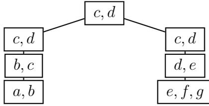
Figure 1: A tree decomposition of the graph in Example 1.
