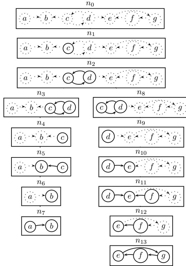
Figure 7: Tree decomposition of  $F$  with subframeworks.
